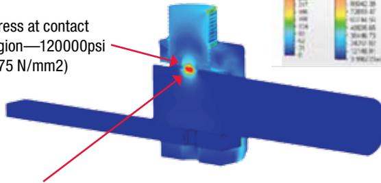
At the contact region between screw and conductor, the stress exceeds the maximum bearing strength.
